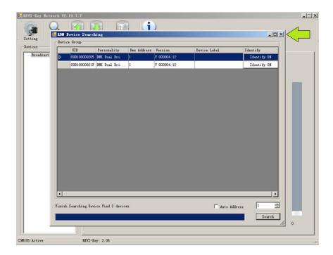
3.) To view and configure the power outputs, select the UID associated to the output ports that need to be configured. – Click Read (this reads all the current configurations saved to the power outputs)
