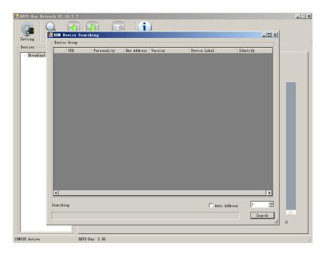
2.) Once the scan is complete all connected devices will appear in the Device Group Window – Close this window.
